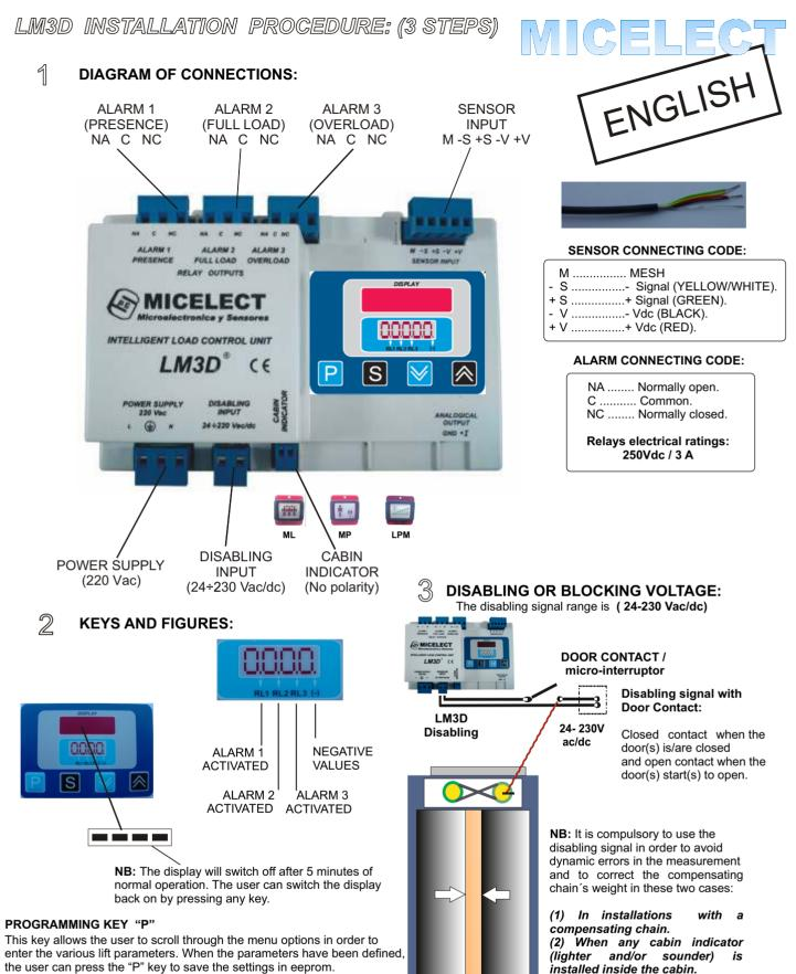
The LM3D must receive a constant blocking signal throughout the entire journey of the lift from the moment the doors are almost fully closed to the moment when the cabin has reached the floor and the doors are starting to open again.
